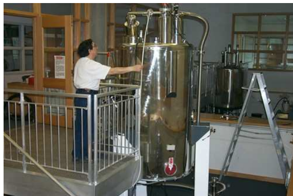
Figure 7: Duke has a world class set of high field NMR spectrometers, including 500MHz, 600MHz, and 800MHz instruments. Shown here is the 800MHz spectrometer, which is currently the state of the art for macromolecular NMR structural determinations.
