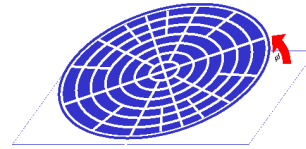
Figure 9: Conceptual design of an actuator array that implements a combined radial-gravity field. Individual actuators are tiled in a circular array pattern. The array is tilted between \phi = 0^\circ and 45^\circ to add a gravity component \delta g with \delta = \tan \phi .
