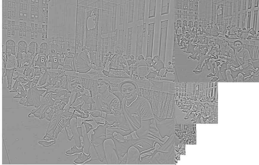
Figure 4: A Laplacian pyramid. Pixel values are positive and negative, and gray denotes zero.
