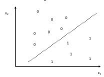
A linear threshold unit always produces a linear decision boundary. A set of points that can be separated by a linear decision boundary is linearly separable.
