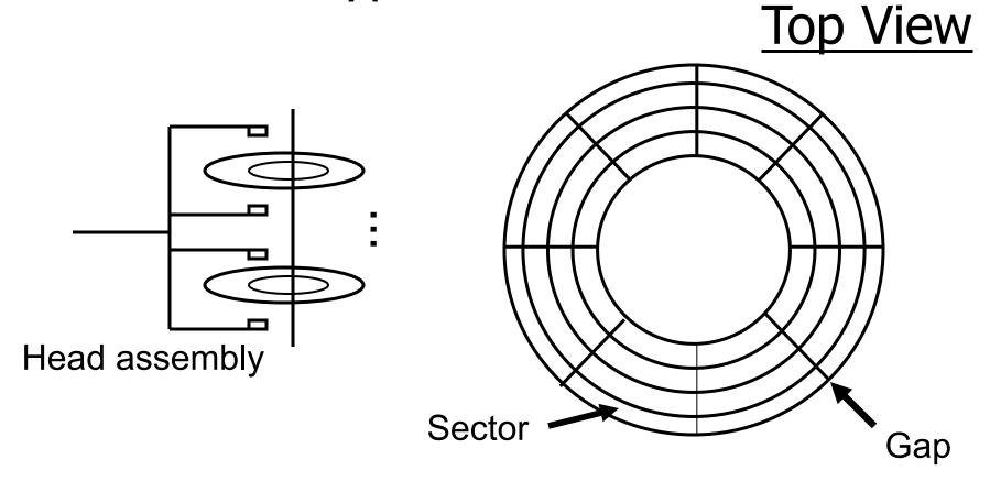
Terms: Platter, Head, Cylinder, Track Sector (physical), Block (logical), Gap
