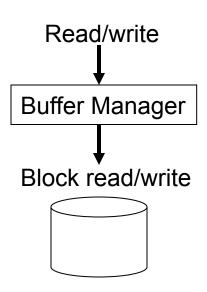
May control memory directly (i.e., does not allocate from virtual memory controlled by OS)
