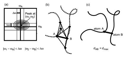
Fig. 3. Three conditions that must be fulfilled by a valid assignment of a NOESY cross peak to two protons A and B in the CANDID automated NOESY assignment algorithm [69]: (a) Agreement between chemical shifts and the peak position, (b) network-anchoring, and (c) spatial proximity in a (preliminary) structure.
