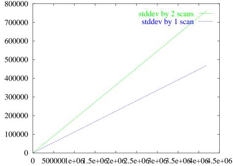
Plot of list size (n) vs. running time (in microseconds) for two algorithms for calculating the standard deviation of a list.
