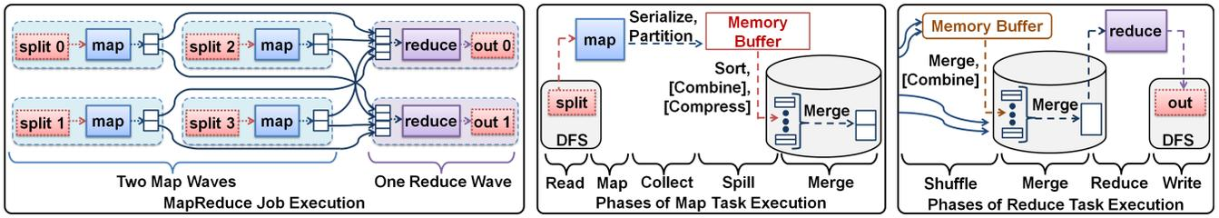
**Figure 4:** (a) Execution of a MapReduce job with 4 map tasks (executing in 2 waves) and 2 reduce tasks, (b) zoomed-in version of a map task execution showing the map-side phases, (c) zoomed-in version of a reduce task execution showing the reduce-side phases.
