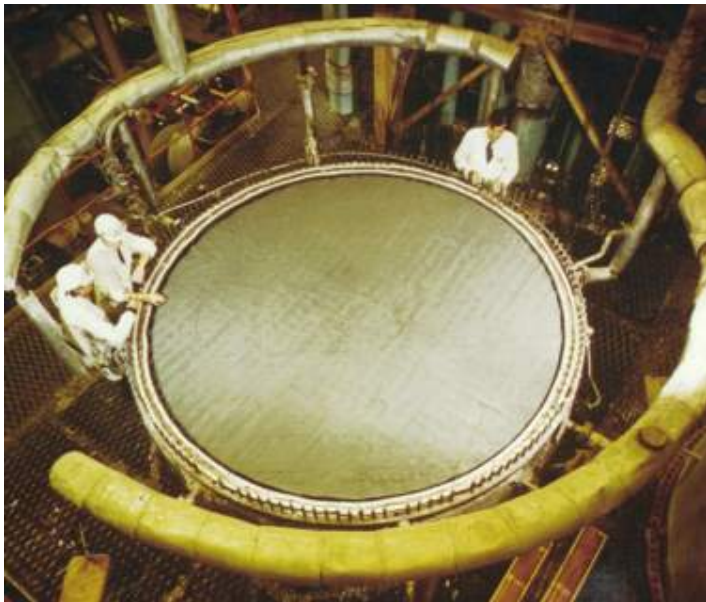
Pt-Rh catalysts used in Ostwald process
