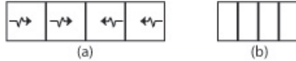
Fig. 2. The Squeeze problem: Expanding cube modules in (a), each of length 1, contract to each have length 1/2 and form the configuration in (b).
