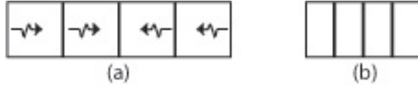
Fig. 2. The Squeeze problem: Expanding cube modules in (a), each of length 1, contract to each have length 1/2 and form the configuration in (b).
