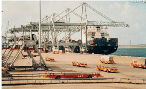
Figure 1: Automated Guided Vehicles in the Delta Port Terminal at Rotterdam [IOANNOU et al. 2000].
