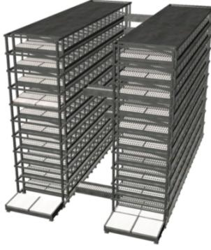
Figure 4: Structure of automated storage/retrieval system (AS/RS) in container yards.
