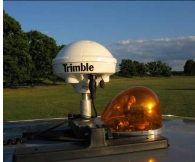
measurements each time a GPS position is received. In trials, dead reckoning was accurate enough to navigate an entire 200 meter course successfully. Parameter estimation techniques allow Prospect Eleven to continually adjust for changes in the car’s state equations. As dead reckoning relies on accurate rotation data from non-slipping wheels, four wheel drive cannot be used unless absolutely necessary.
