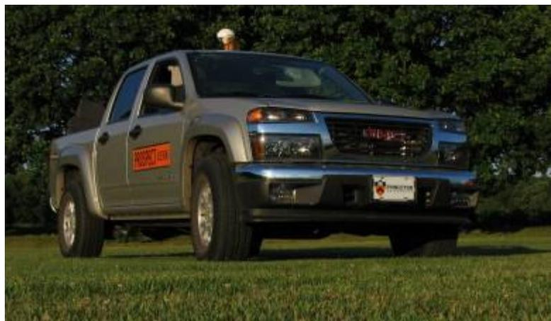
vehicle's suspension and wheels remain stock. It has a wheelbase of 3.2 meters, and a turning radius of 13 meters. The back seats were removed to provide space for vehicle control systems, but the front seats were left intact. Prospect Eleven remains fully human-drivable.
