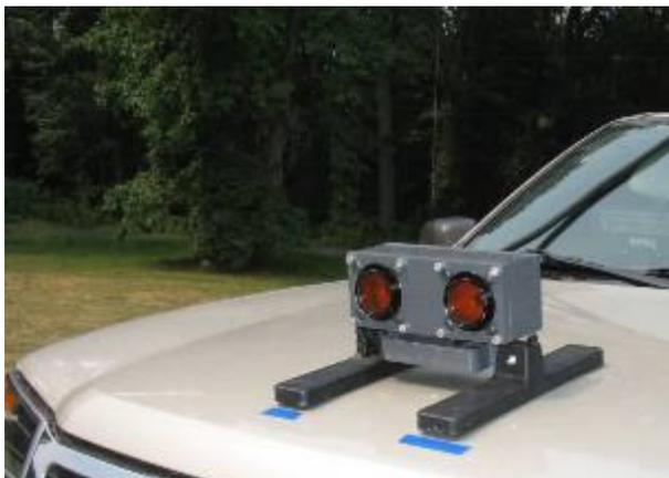
stereo camera mounted on the hood of the vehicle. Obstacles can be reliably detected at 50ft, with a horizontal field of view of 70°. Obstacles below 30cm in height are generally not detected until they are very close, due to the limits of the stereo image. The detection algorithm searches for deviation from a dynamically-computed ground plane. Stereo
