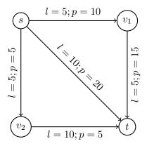
Example: For the graph on the left, there are three paths from s to t. The path we are looking for is  $(s, v_1, t)$ , with length 10 and maximum slope 15. The reason why  $(s, v_2, t)$  is bad is that it has total length 15, so it is not a shortest path. For the path (s, t), even though it has the same length 10, its maximum slope is 20, which is worse than that of  $(s, v_1, t)$ .
