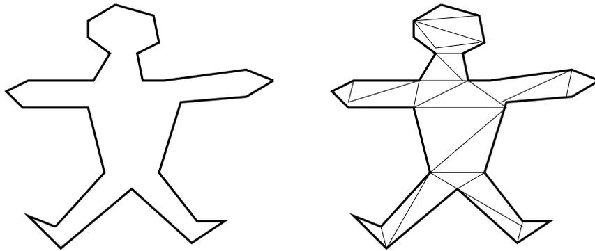
Triangulation is an important first step in many geometric algorithms.
