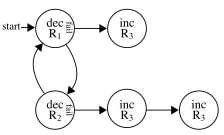
A register machine comparing the value of register  $R_1$  to  $R_2$ . If  $R_1 \le R_2$ , then it outputs 1 in register  $R_3$ . If  $R_1 > R_2$  then it outputs 2 in register  $R_3$ .
