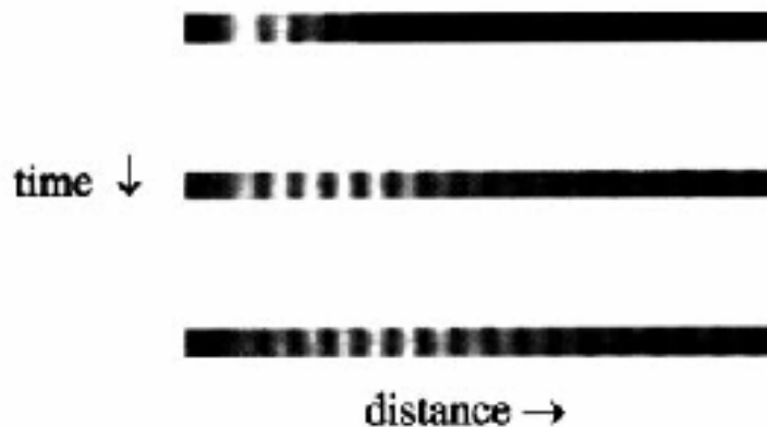
Fig. 3. Three images are shown from a typical experiment using a device with 2- \mu\text{m} electrodes and a 0.7-Hz switching frequency to transport a rhodamine-labeled DNA 50-mer. These images were saved during the trapping phase of the cycle, and fluorescence maxima are clearly seen from DNA molecules captured on the positive electrodes. At the start of the experiment, the DNA oligomers are focused on left-most three electrodes. As the potential cycles between on- and off-states, the packet moves to the right and broadens.
