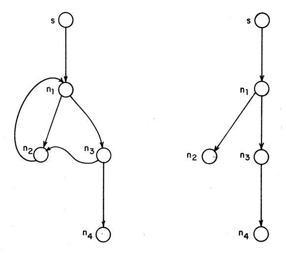
Figure 1.3. A flow graph and its dominator tree.
