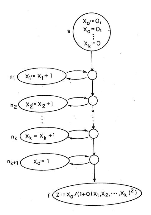
Figure 1.4. The control flow graph FQ.
